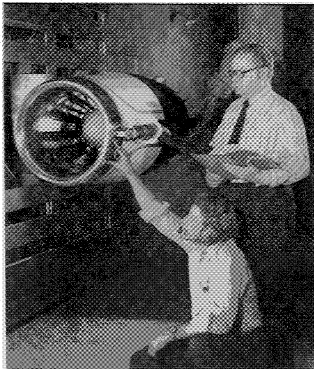
Fig. 1 0.508-m-diam fan/inlet installed in V/STOL tunnel.
